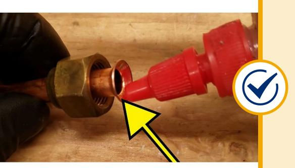
Apply **compatible** refrigerant oil to the **face** and **never the threads**
